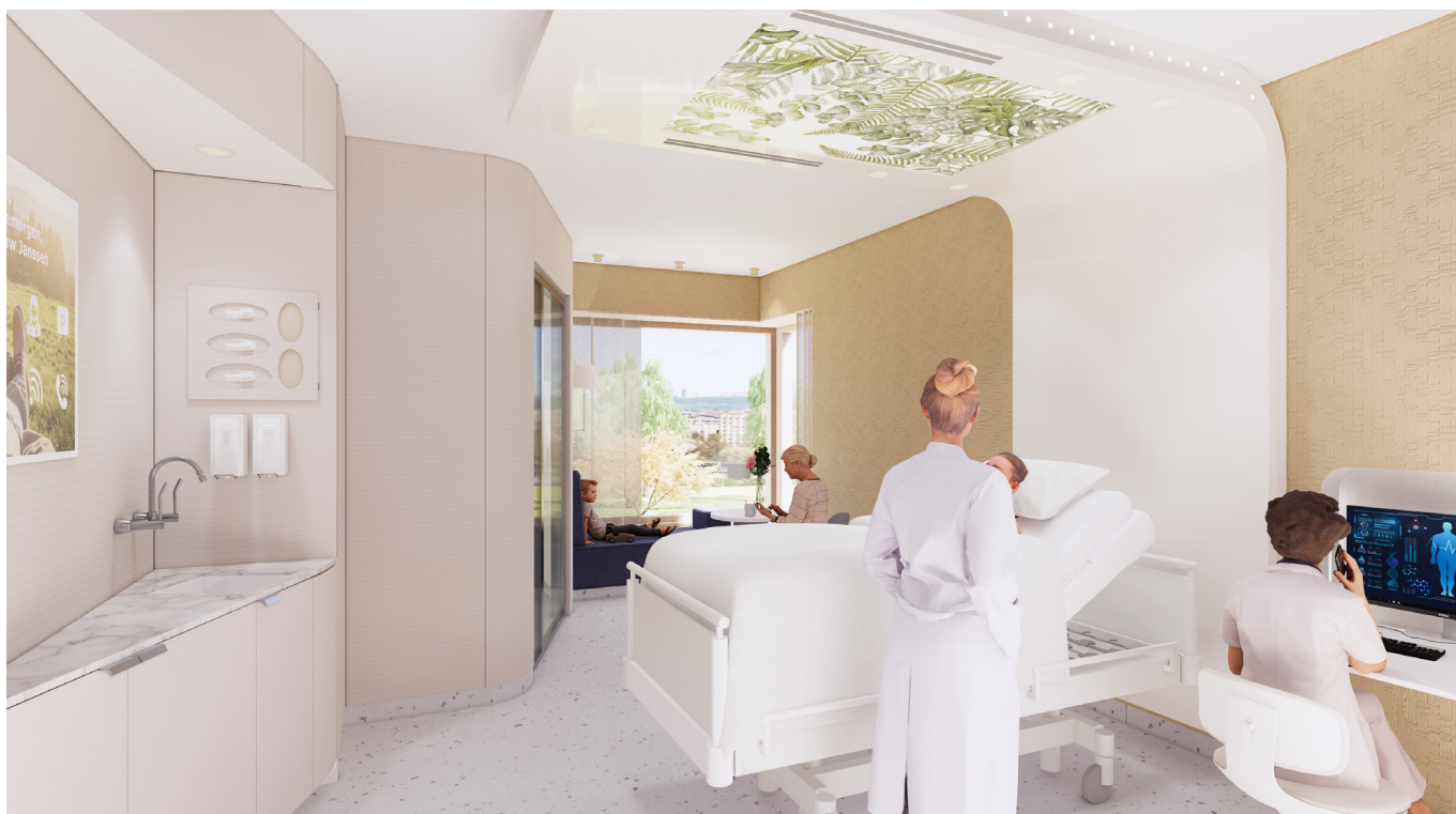
Medium care room in the nursing ward with “rooming-in” functions and decentralised post/supplies and technology around the bed
